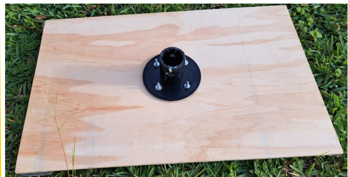
Close-up of the underside of the 5 ply top. The screw heads are countersunk to leave a smooth surface on top
